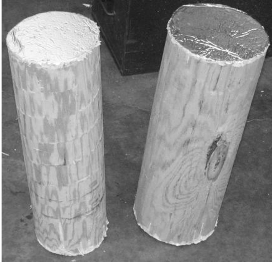
Figure 5.1 Pole samples with urethane adhesive and aluminum foil
