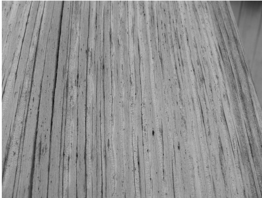
Figure 2.2 Surface checking on flatsawn southern pine lumber
