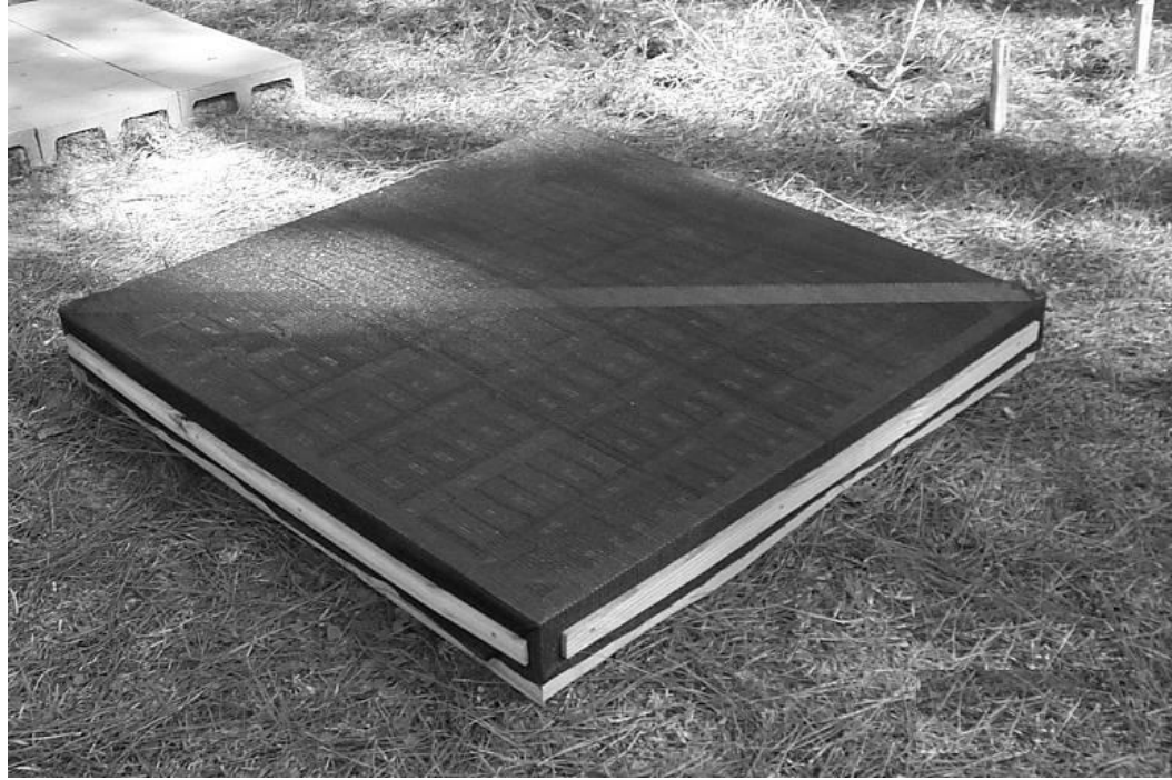
Figure 4.1 Ground decay test setup; samples are beneath the screen cover
