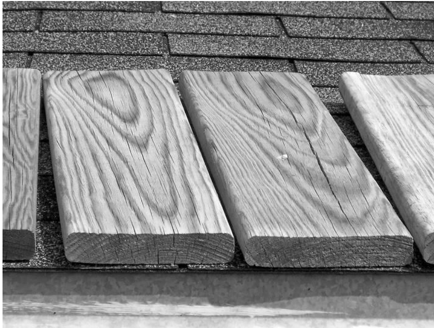
Figure 3.3 Roof test setup showing 32 mm x 140 mm decking board sections
